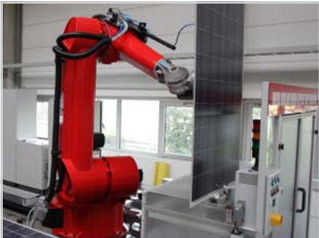
The laminate is guided directly at the applicator by a robot. Application of adhesive tape, edge-folding and application of the lubricant is done in one step.
