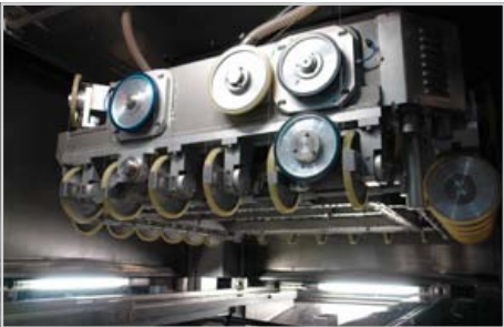
Bricking with Diamond Wire
